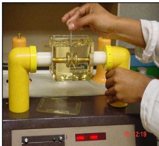
Figure 3: — Typical dielectric strength test cell
