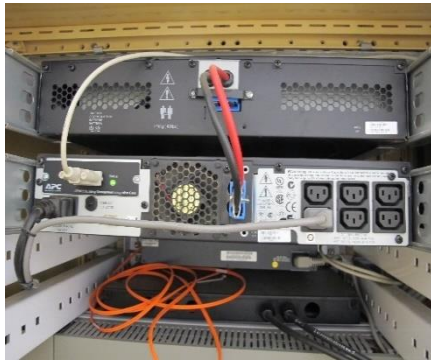
Rack mount UPS with additional battery pack
