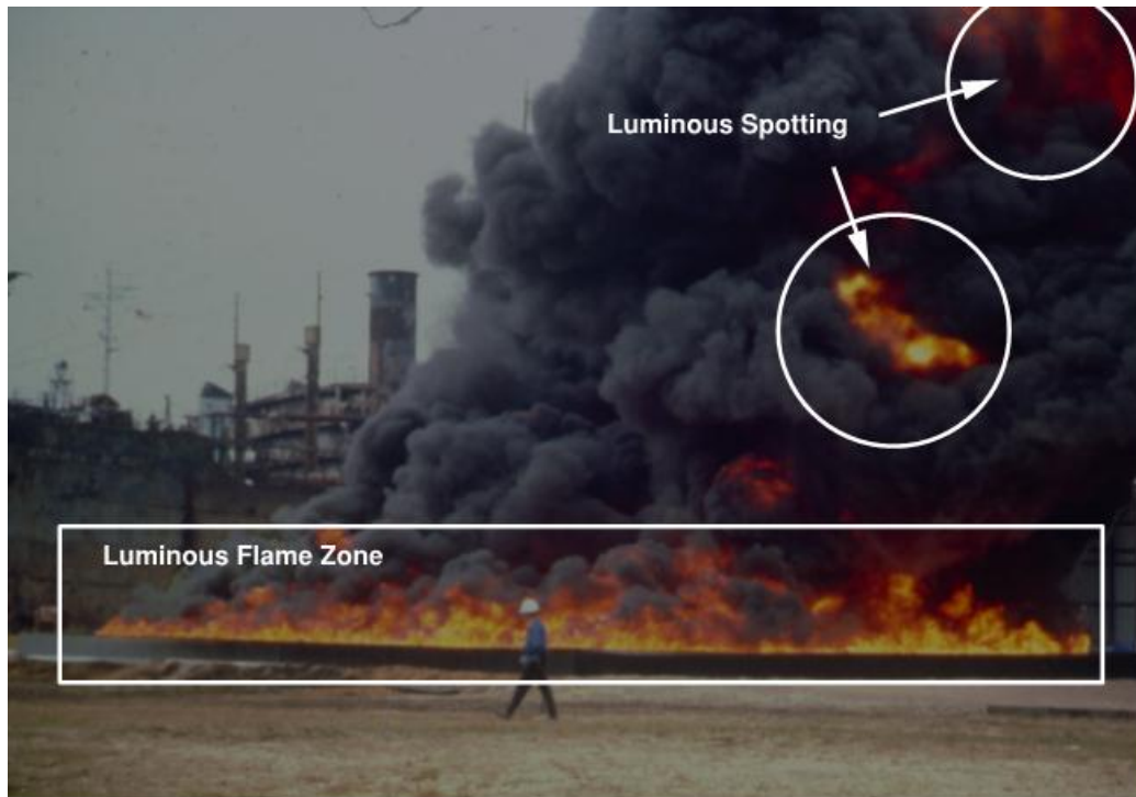
Figure 5: Large hydrocarbon pool fire showing luminous flame region near the base of the fire [112].
