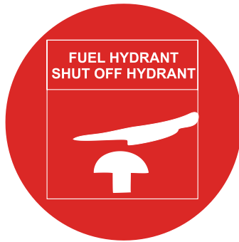
Emergency stop for fuel hydrant system
