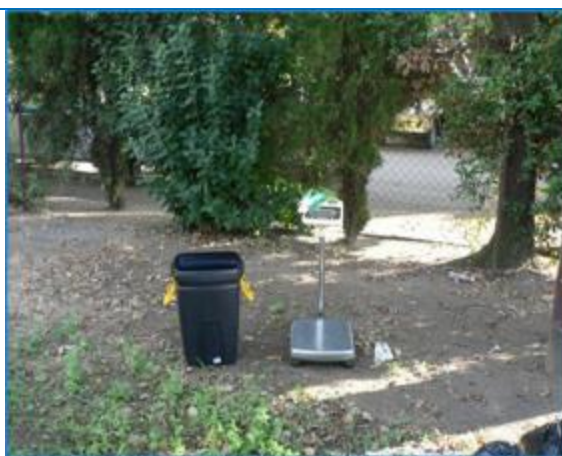
Figure 8: Standard 85L bin and Scale used
