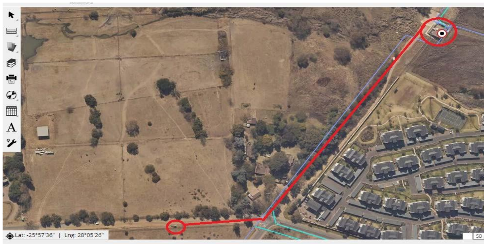
Figure 1: Cable path. The big red circle is the pump station and the small red circle is the Eskom kiosk
