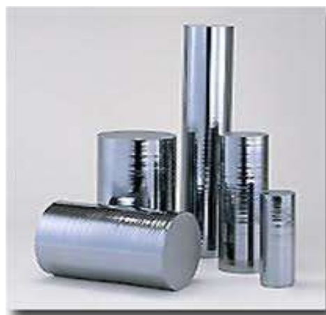
Figure 3: The ingot diameter varies from 128 mm to 152 mm, with a length of 600 mm.
