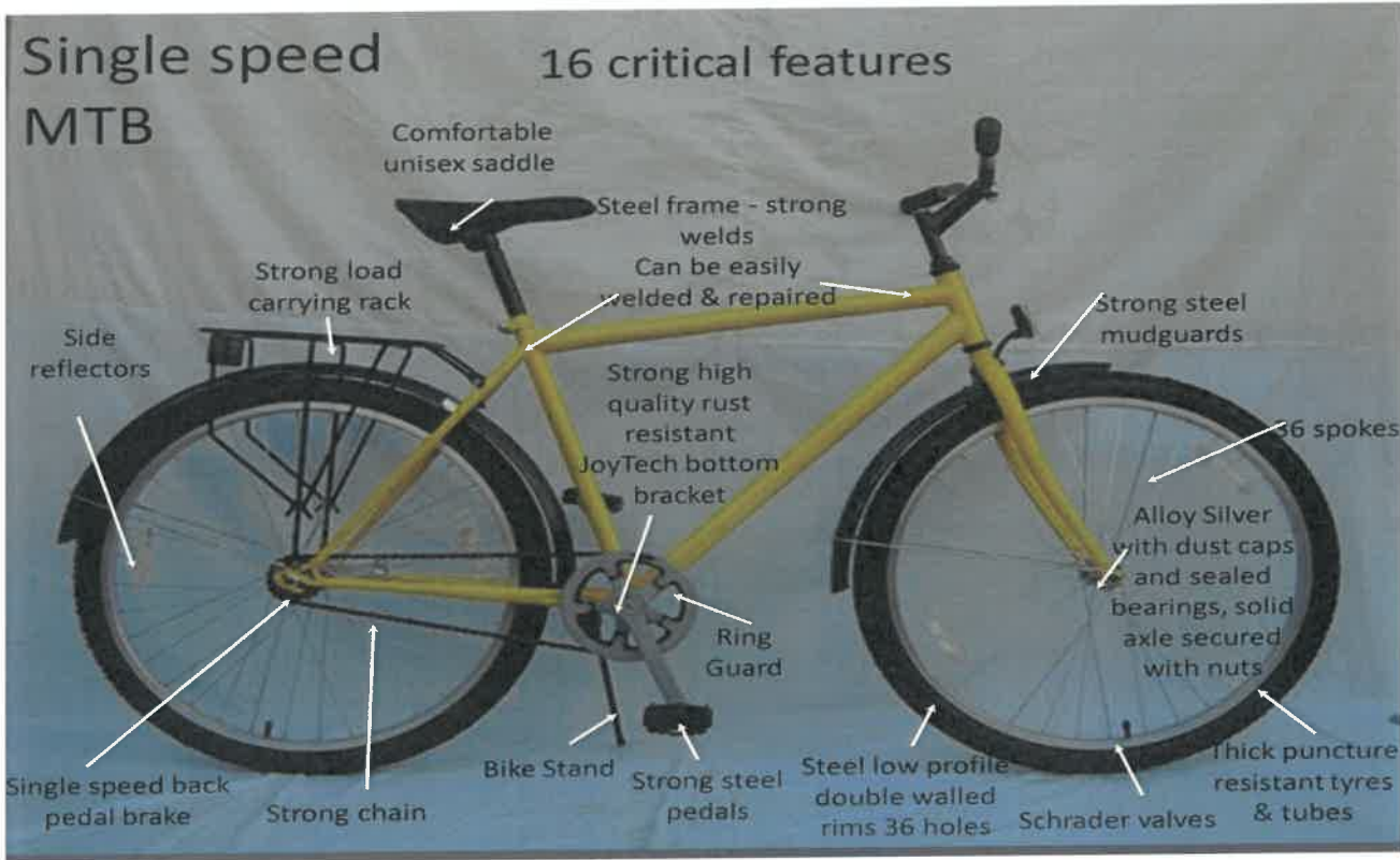
FIG 1: BICYCLE SPECIFICATION: SHOVA KALULA BICYCLE
