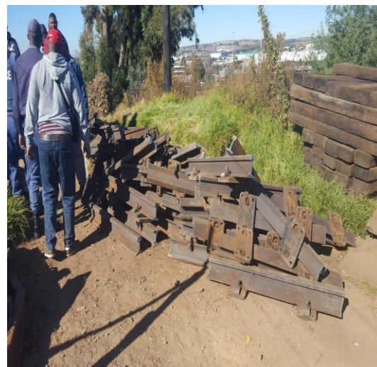
Fig 2.2: Stolen turnout components and sleepers
