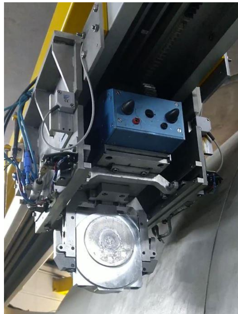
Figure 4: Left: Target holder and target capsule (fits into target holder), Right: Target holder on trolley docked in end station,
