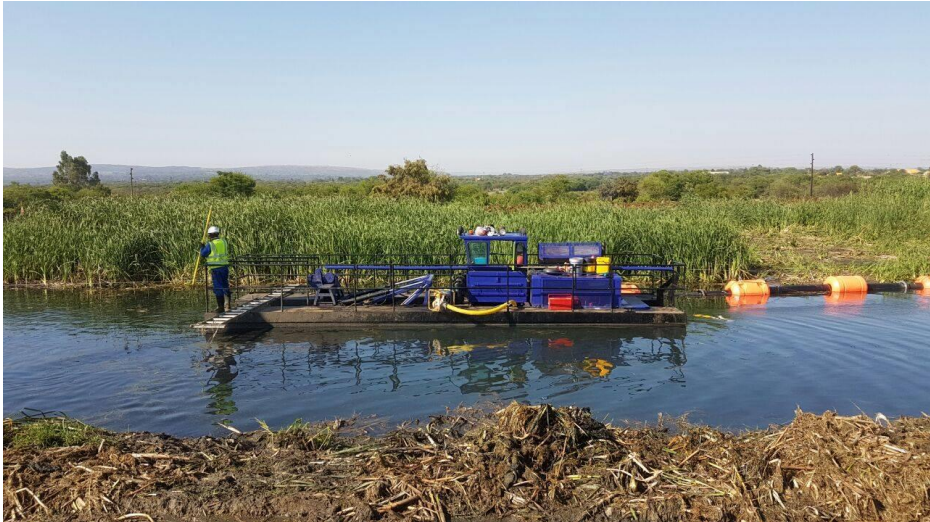
Figure 4: Example of a floating barge
