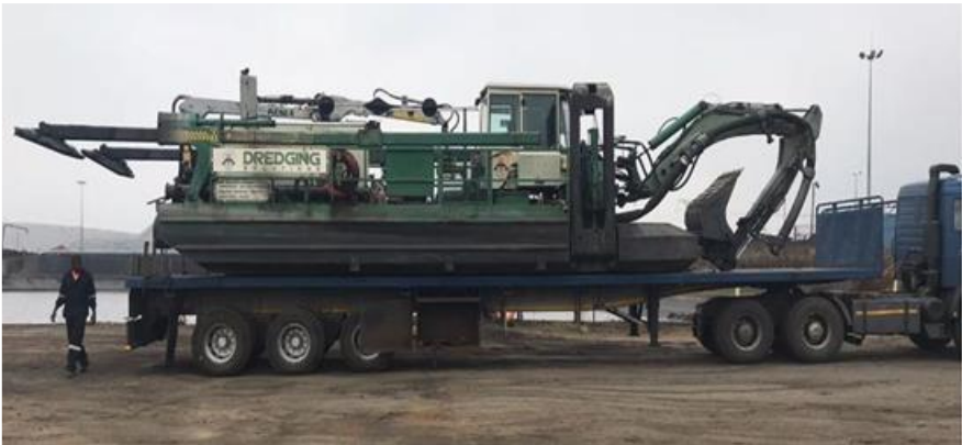
Figure 3: Amphibious multi-purpose dredger, showing ease of transportation to site (from Bosch projects, 2022).
