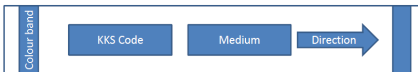
Figure 27: Pipeline label (Greater than 35mm)
