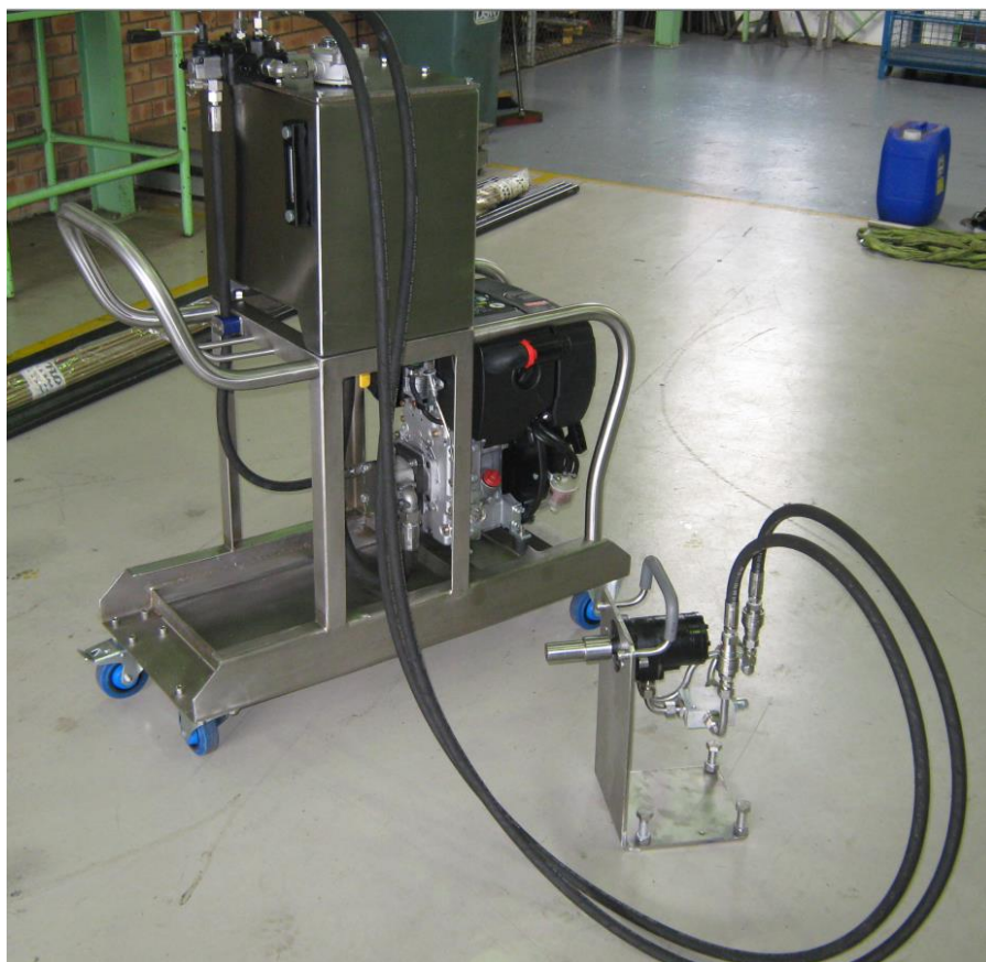
Ntshingwayo dam: Radial gates Mobile diesel driven hydraulic unit
