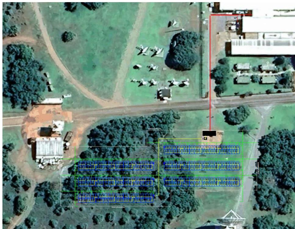
Fig 1: Plant 1 – 200kWp. Coordinates: -25.887745, 27.707386, Area: 748m<sup>2</sup>
