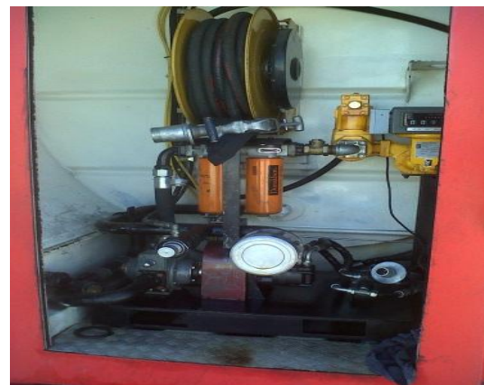
Figure 34: Fuel bowser pump arrangement
