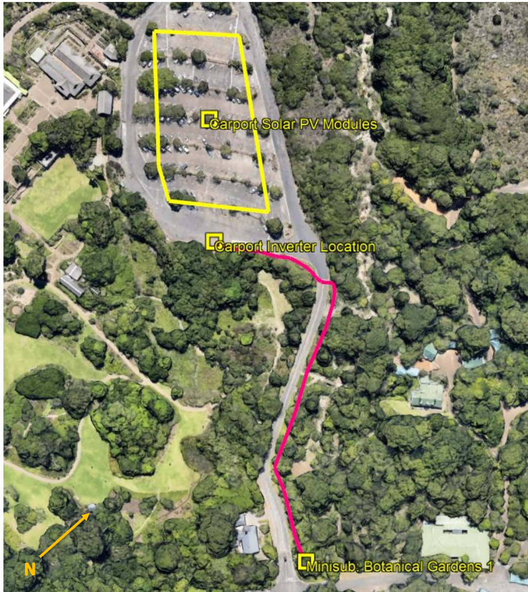
Figure 4-6: Cabling routing from Carport PV inverters to Minisub: Botanical Gardens 1
