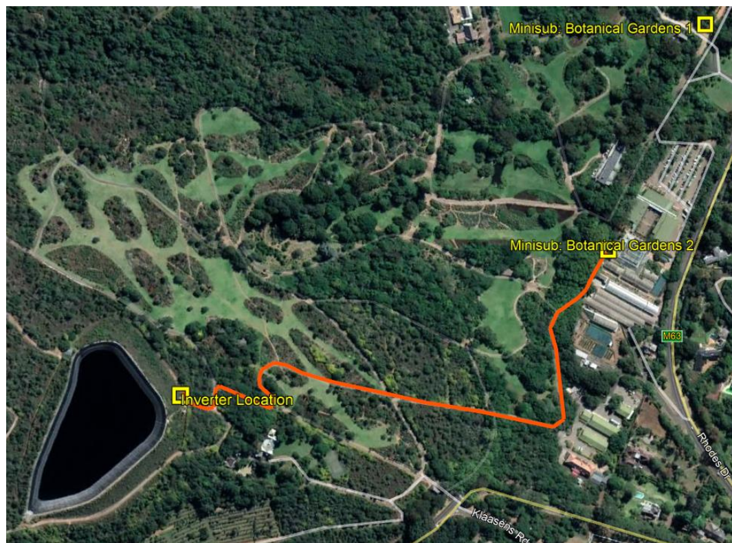
Figure 4-2: Cabling routing from PV inverters to minisub: Botanical Gardens 2
