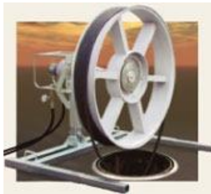
Figure 4: Roller cable off the spool to prevent twisting
