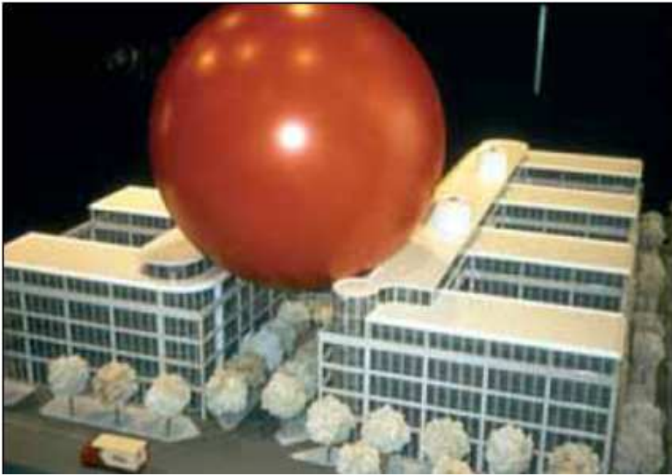
Figure 8: Illustration of the rolling sphere method [18]
