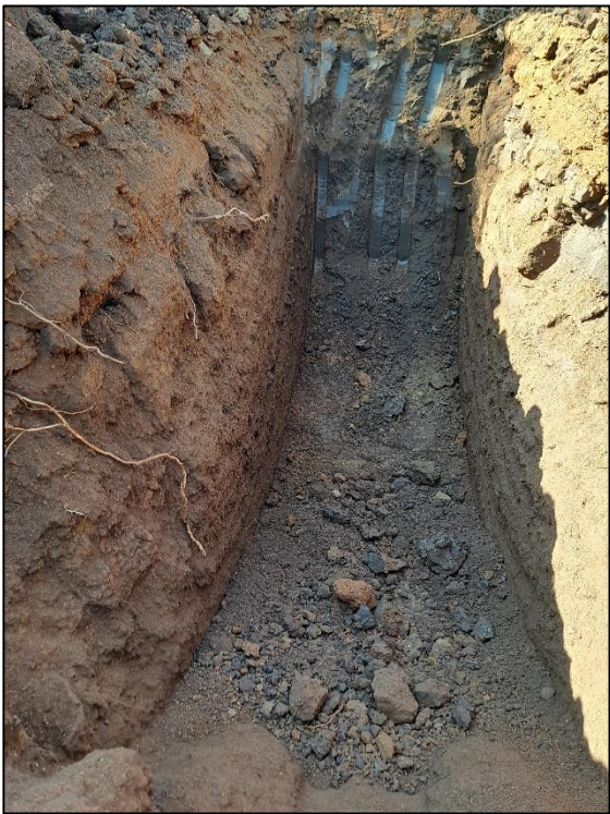
Plate 3 (Left): Deeper transported finer grained soils at TP1 and TP2. Plate 4 (Right): Sporadic rock at surface between TP5 and TP6. Note TP6 with weathered mudstone from surface throughout cut extent.
