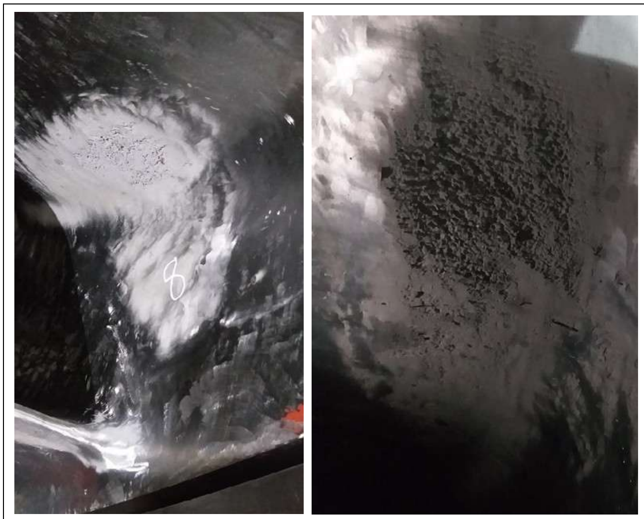
Figure 7: Turbine blade low pressure area cavitation
