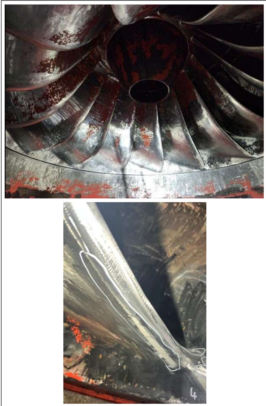
Figure 6: Turbine blade trailing edge cavitation
