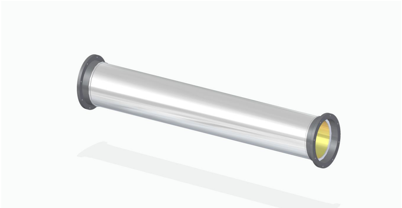
Figure 2: Three-dimensional drawing of the ceramic beam pipe with flanges.
