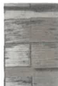
Plate 9 Bond quality 80% in visual linear scale
