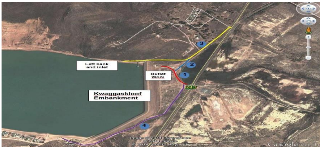
Figure 3: Plan view of Kwaggaskloof embankment (Google Earth, 2013)
