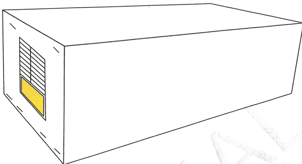
Figure 3 – Lid component of telescopic cardboard box (assembled and ready to serve as the lid of a container for storage of finished goods)
