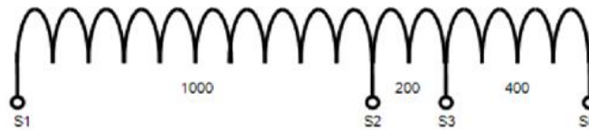
Figure 5: Tapping Arrangements for Multi-ratio 1/1 600t bus zone cores
