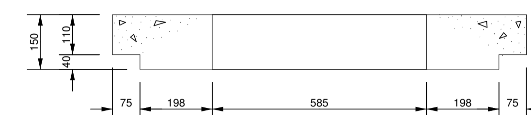
SECTION OF CIRCULAR COVER SLAB
