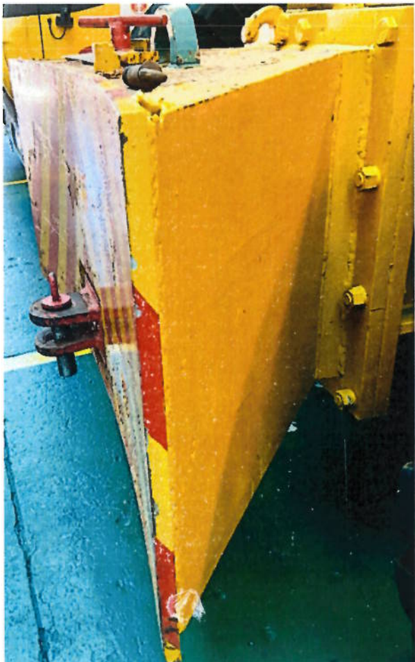
Figure 4: Side view of Front push plate.
