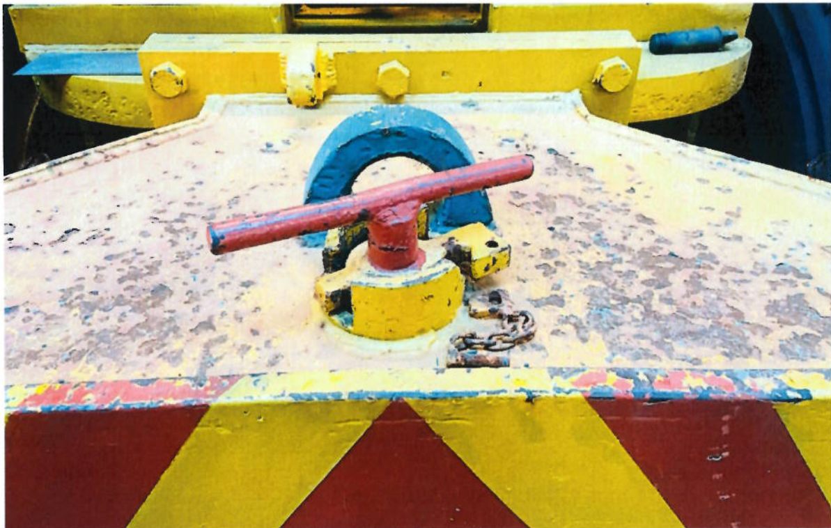
Figure 6: Top view of front push plate
