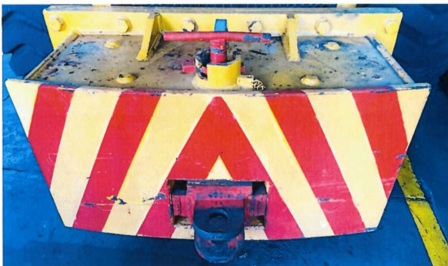
Figure 3: Front view of rear push plate
