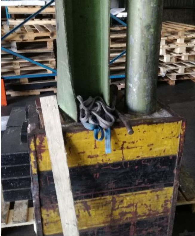
Figure 20 Sheared steel column flange
