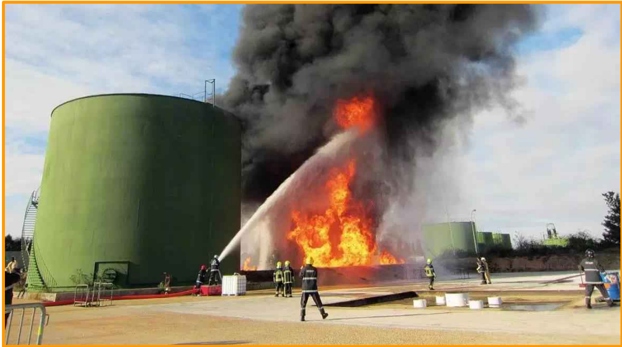
Figure 3.2: Illustration of pool fire (also showing smoke dispersion)
