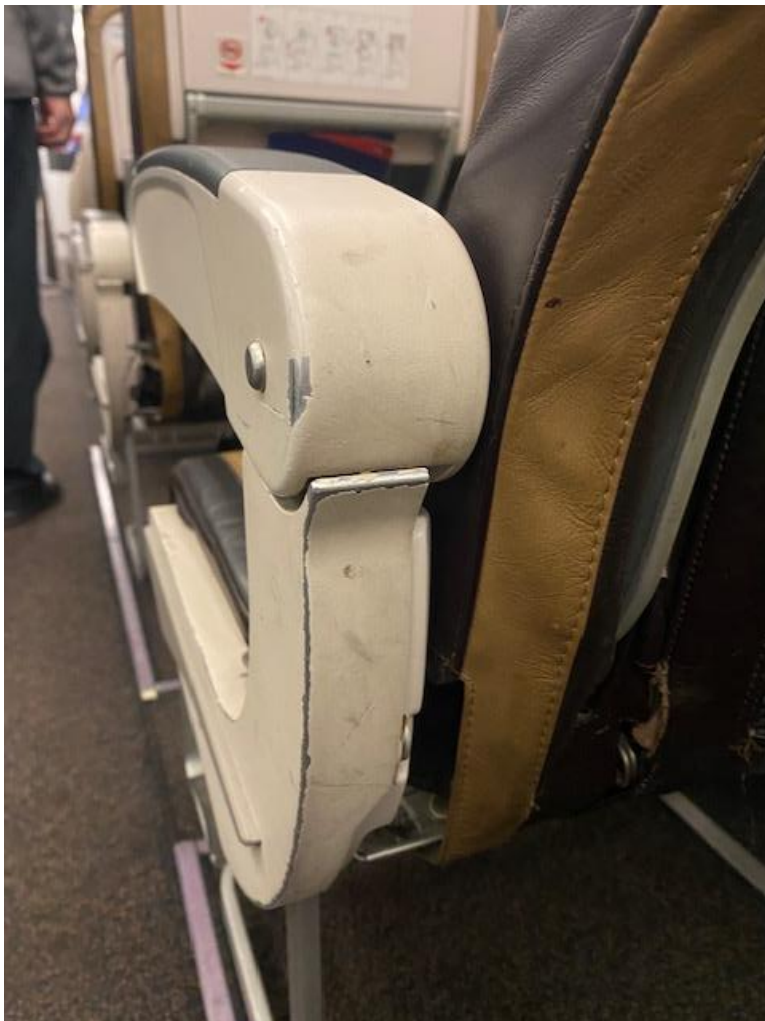
Damage to paint
