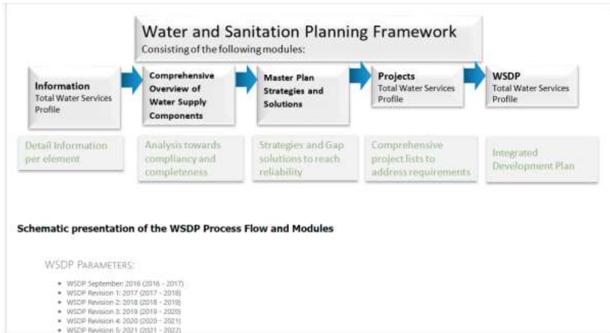
Figure C1: WSDP Modules and Process Flow [Per Department of Water and Sanitation (DWS)]
