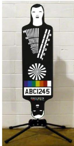
**Figure D.1: Rotakin Test Target**
