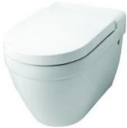
Vaal Sanitaryware vitreous china "Energy" 90° outlet back inlet closed rim wall hung pan, with quality thermostet soft-close seat (code: VAA-439500WH) and DP Flushfit pan collar (or equivalent). Flush volume 6/3 litres, subject to the pan being installed with a cistern providing an effective 6/3 litre flush volume.
