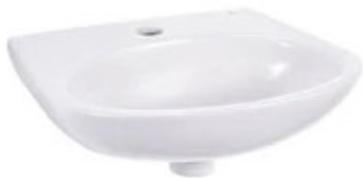
Cobra Welcome Medium round wall hung basin (Product Code: 709100WH). 430mm long x 390mm wide. 1 x pre-punched tap hole in the centre of the basin. Wall fixing set & installation manual included.
