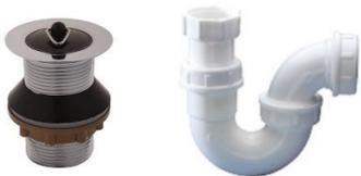
Cobra unslotted basin waste with 62mm diameter flange and 75mm long shank, and 1 ¼" BSP male outlet connection. du Bois 40mm PVC trap.
