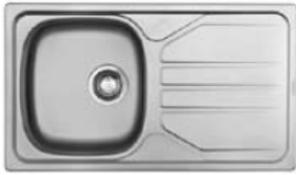
Franke Nouveau Inset Sink model NVN611 Single End Bowl Sink Drop-on Sink (Product Code: 811023), 800 x 460mm Single End Bowl S/S grade 304 18/10, 1,6 mm drop-in sink unit. Unit to be manufactured from Austenitic Stainless Steel with a satin finish, and supplied complete with 90mm basket strainer waste fittings. Sink to be fitted to kitchen counter top.
