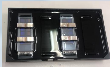
Figure 2: After DNA extraction, the DNA is genotyped using the Illumina Chicken 60K Beadchip. Figure 2 depicts the wash step of the genotyping protocol of a Chicken 60K Beadchip.
