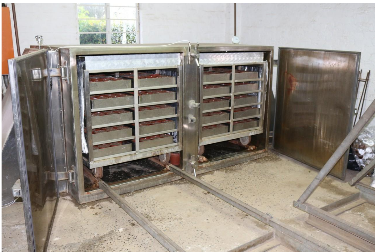
Figure 2. Open, loaded pasteuriser with one set of trolley tracks lowered.
