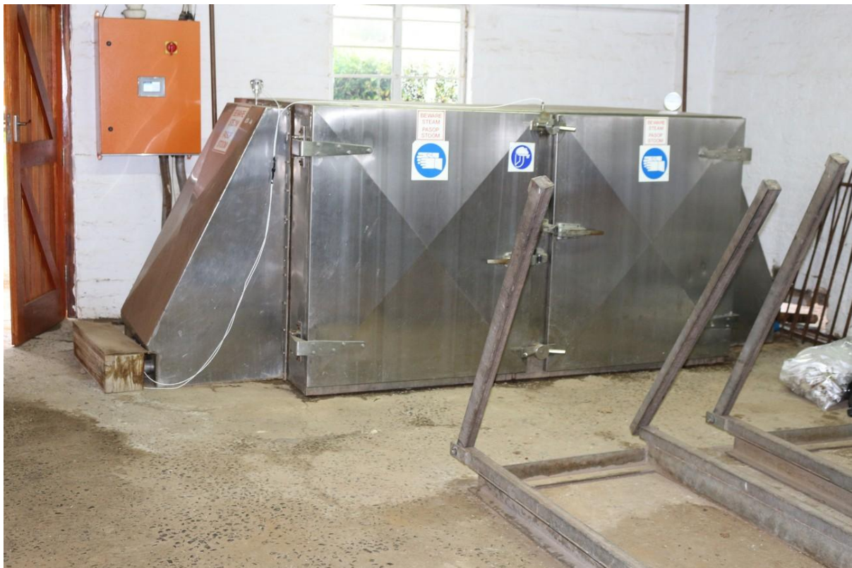
Figure 1. Closed pasteuriser with trolley tracks raised.
