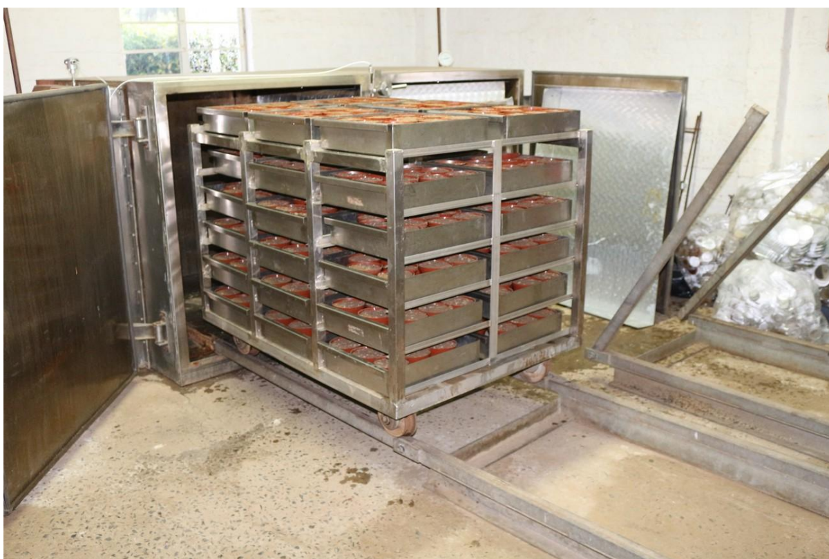
Figure 3. Open pasteuriser with one trolley pulled out onto the tracks. The trolley is loaded with steel trays containing 13 mm diam. pots with soil.
