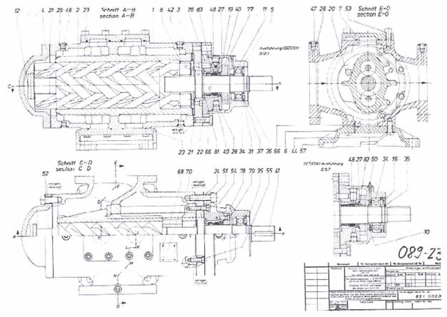
Figure 1: A typical positive displacement 3-rotor screw pump.
