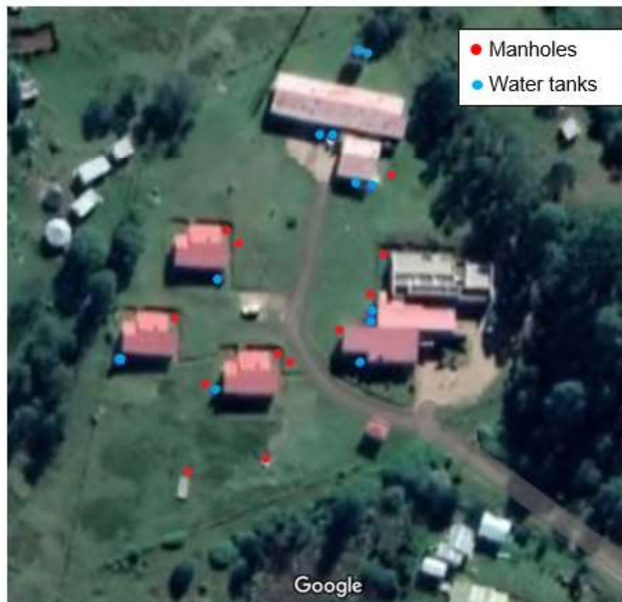
Figure 4: location of manholes and water tanks
