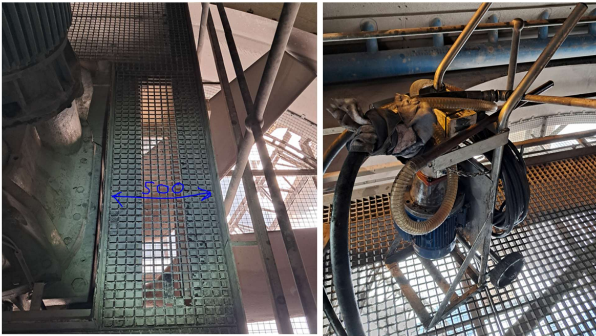
Figure 2: Maximum width restricted by 500mm passage. Existing trolley.
