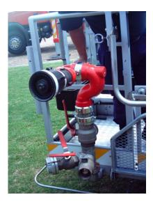
A water monitor shall be connected onto the piping system and placed at the front of the cage on the right hand side just outside of the railing. The monitor shall be made of a suitable material and fitted with jet/fog nozzle with a nominal capacity of 3800 l/min.
