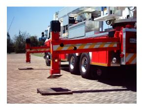
4.3.1 The stabilising system shall consist of four hydraulically powered outriggers mounted in their
