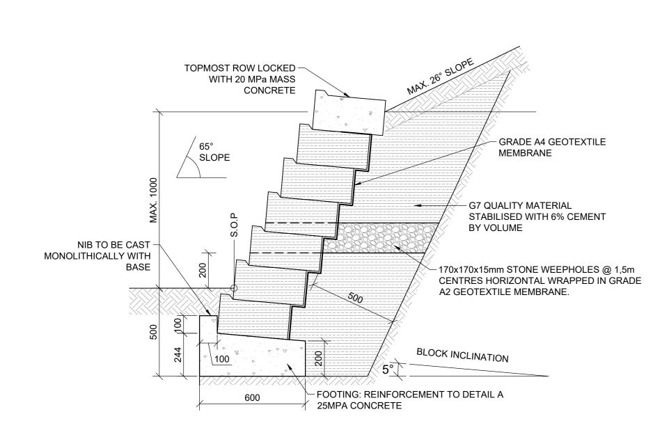
TYPICAL SECTION SHOWING DRY-STACK RETAINING WALL (>0m TO 1m EXPOSED HEIGHT)
