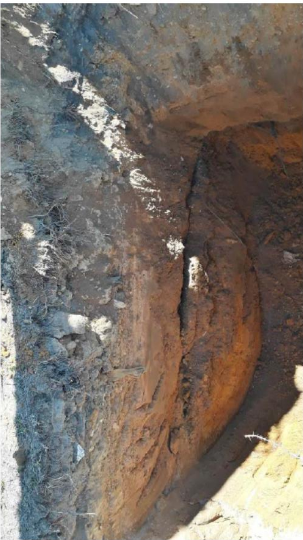
Photo 6 – View of subsoil profile as exposed in trial hole 3, note significant deposit of fill as well as slope instability due to saturation .
