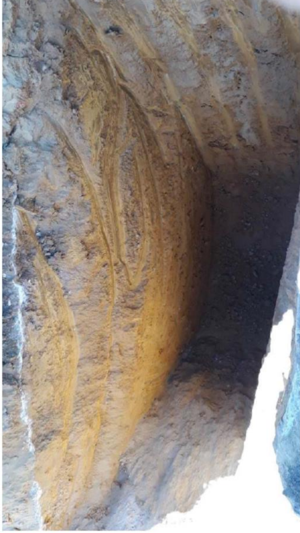
Photo 2 – View of typical trial hole profile comprising predominately naturally transported soils as encountered in trial holes 1&3.
