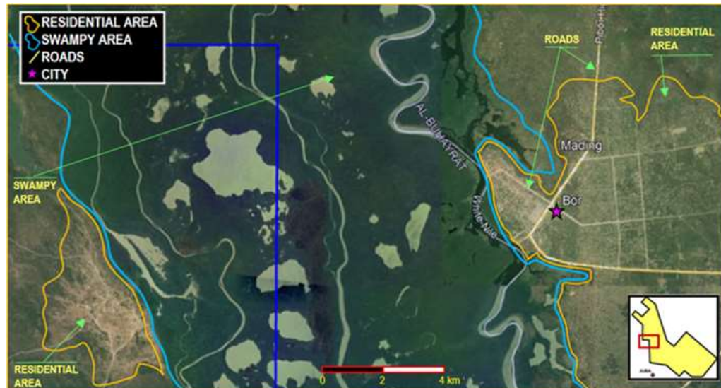
Figure #2: Satellite image of a portion of the area that will be covered by the 2D seismic survey. The survey inspecting will serve to determine obstacles of natural and man-made origin. These obstacles must be considered in the final shooting plan.
