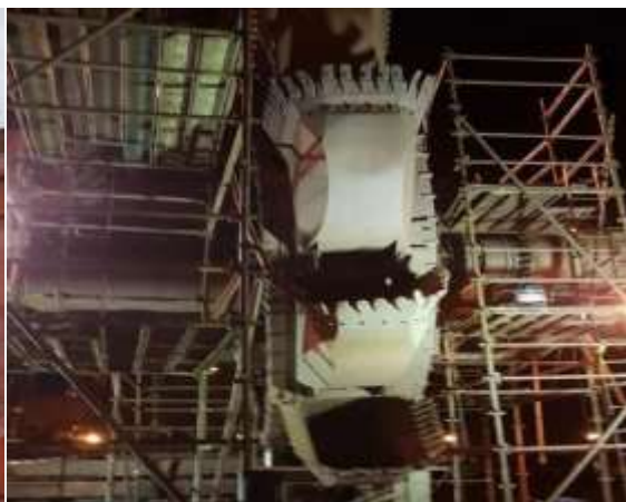
Picture 2: Bucket wheel repairs
