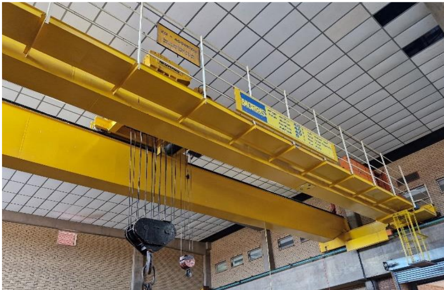
Figure 1: Picture of the 40T Crane at 4 Engine Room Loading
