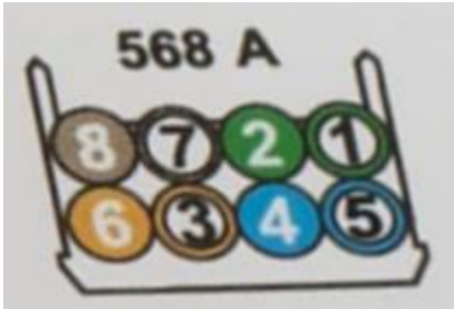
Figure 5-2-3: Connector Colour Coding on Sticker
