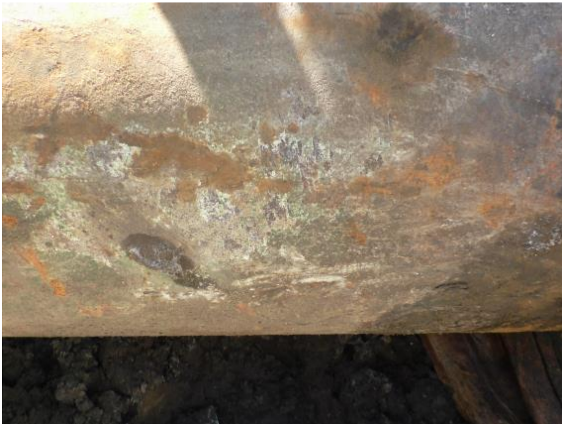
Excavation at leak site. Epoxy coating damaged, no pitting. White corrosion product.
