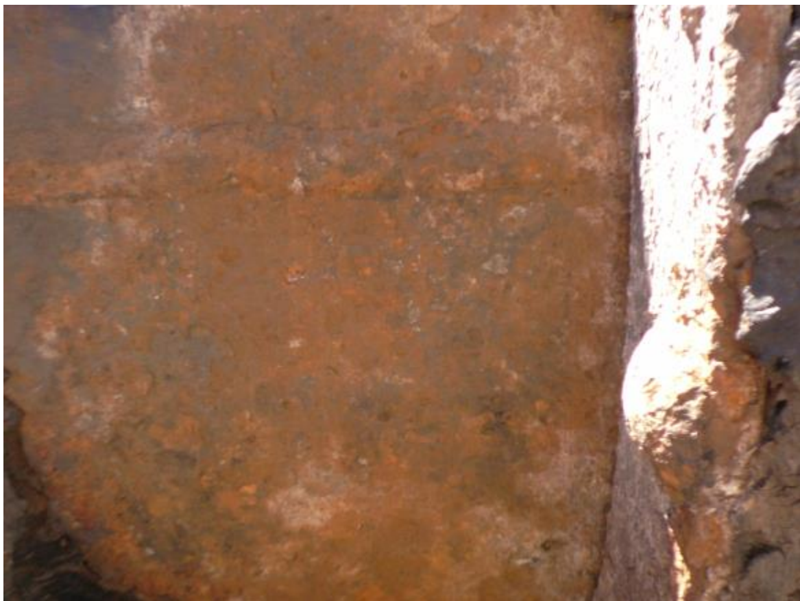
Excavation at defect D55. Pitting area B.
