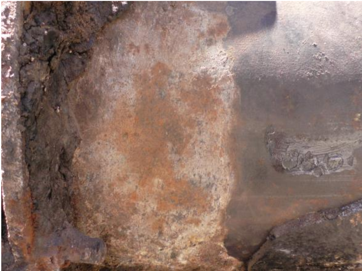
Excavation at defect D55. Pitting area A.
