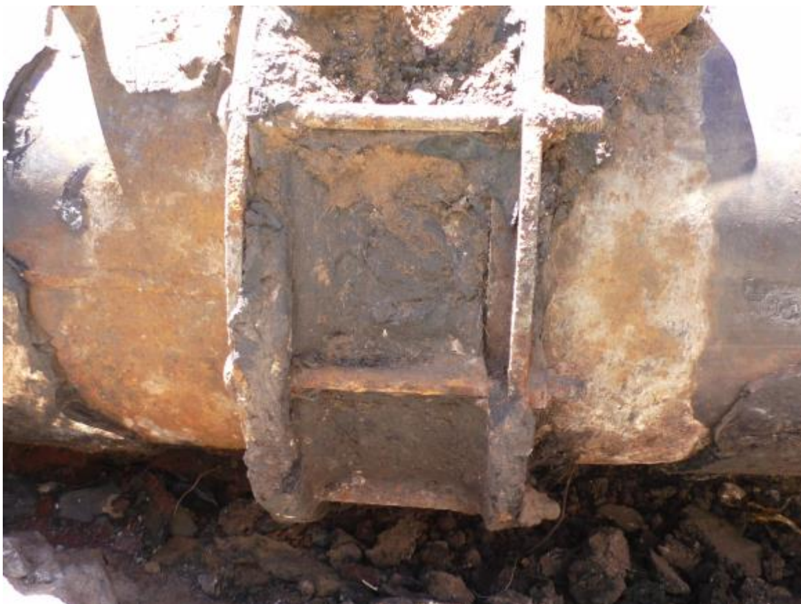
Excavation at defect D55. Pitting area A (right), B (left). Note the rusted bolts.
