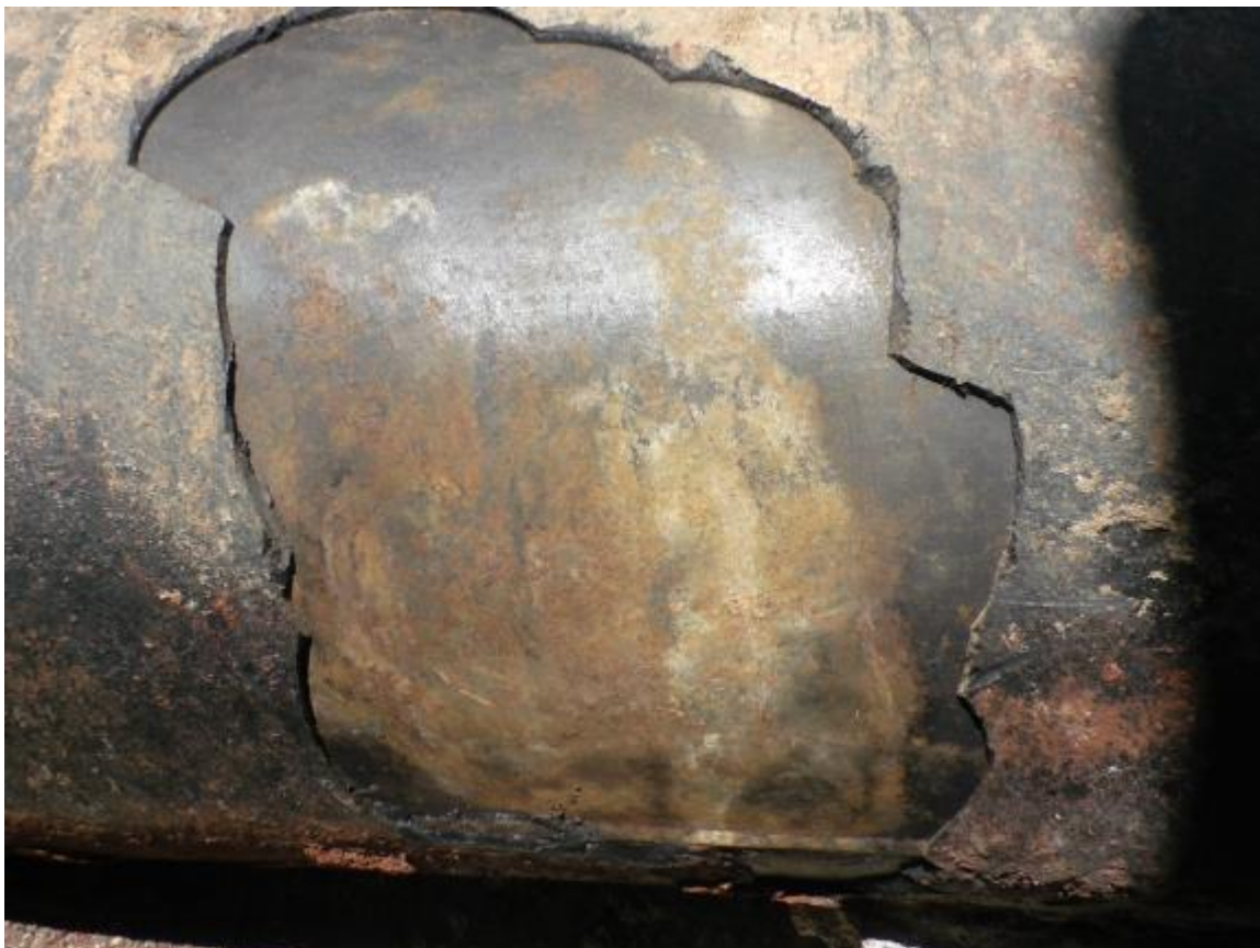
Excavation at defect D10 pitting area
