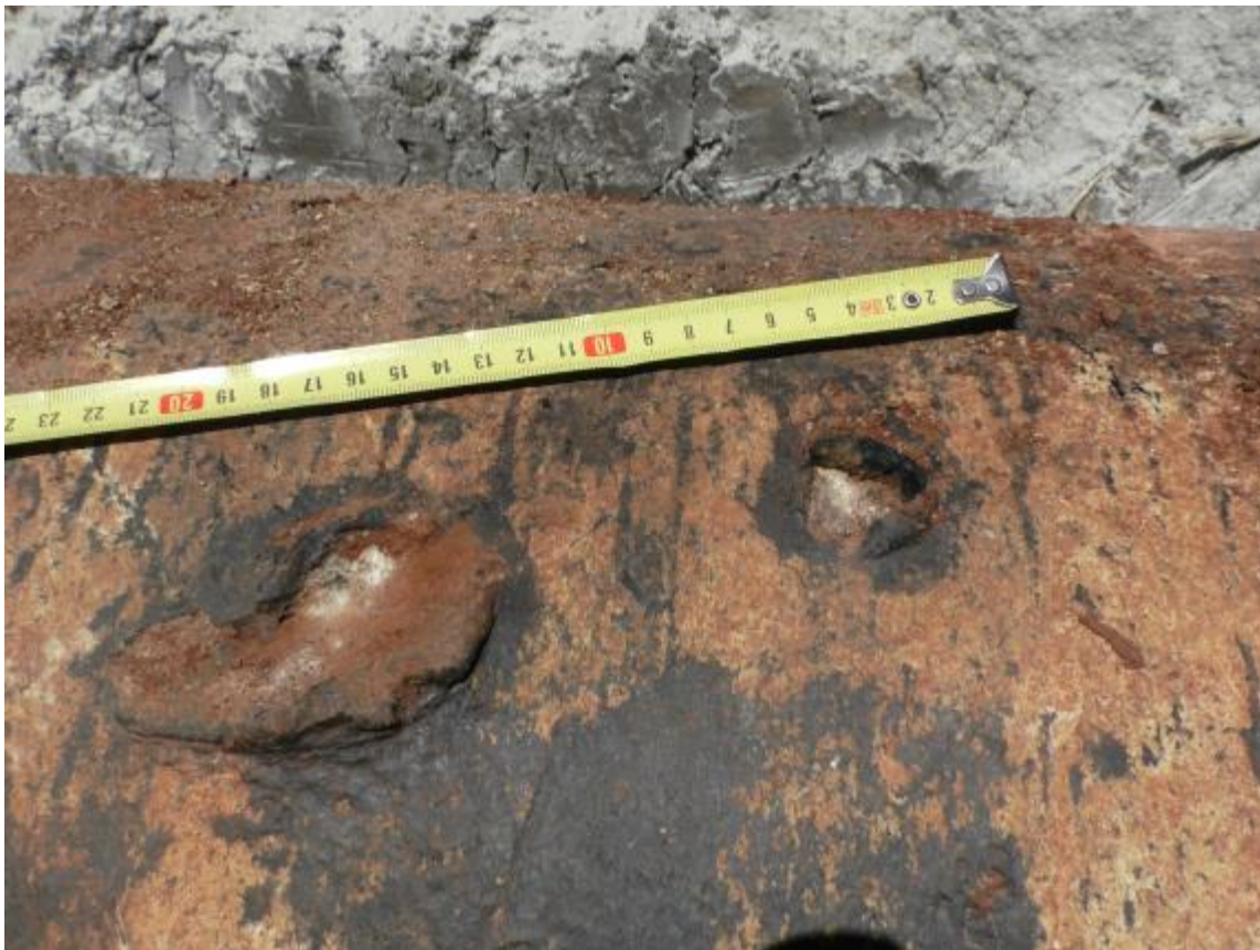
Excavation at defect D10 coating damage. Note the white corrosion product
