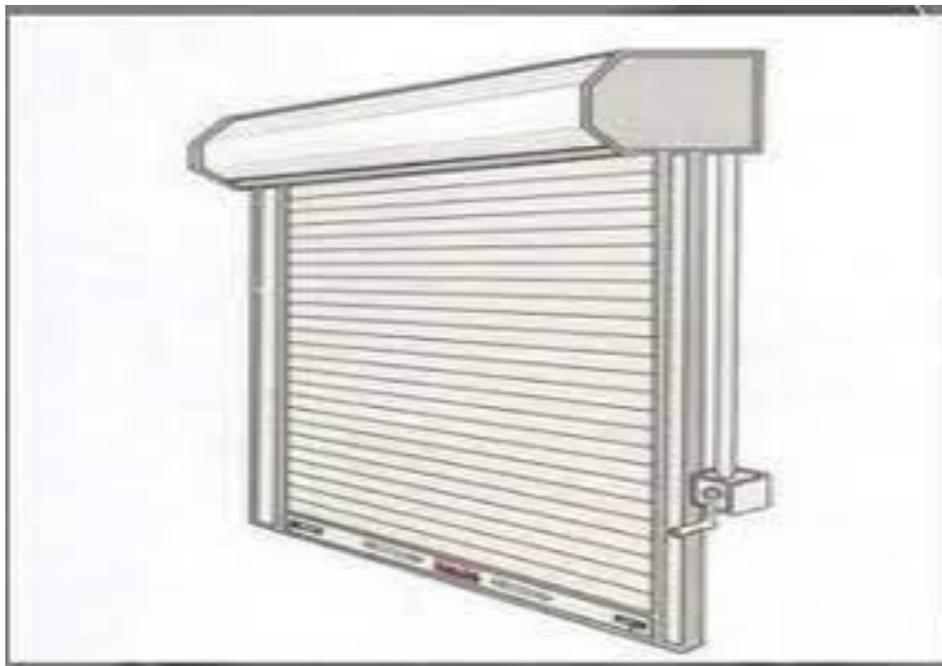
The Roller Shutter Door operates vertically. The entire curtain (heavy duty barrier) rolls up around a barrel above the door. This would not be possible without the aid of a counterbalance springs.
