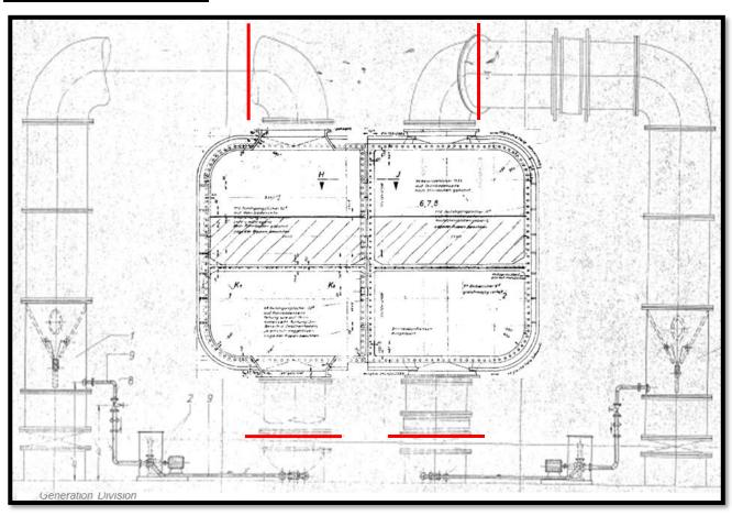
Figure 1: CW Ducting Blanks (Indicated in Red)
