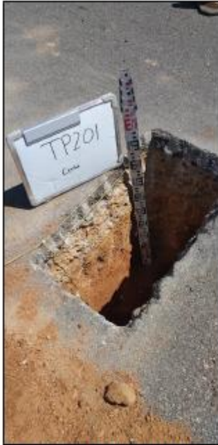
Photograph 1: Material Encountered in TP201 (Centre)
