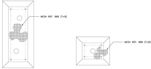
ROOF PLAN-REMOVABLE PANEL REINFORCEMENT DETAILS
